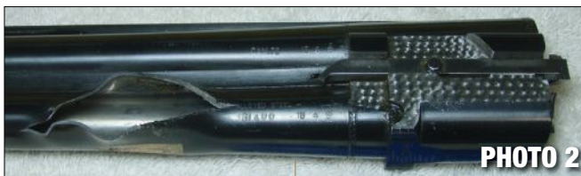
▲ Photo 2: A burst barrel.
