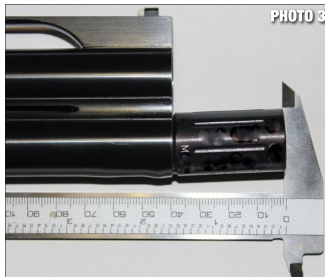
▲ Photo 3: A bad choke tube install job left this barrel bulged.
