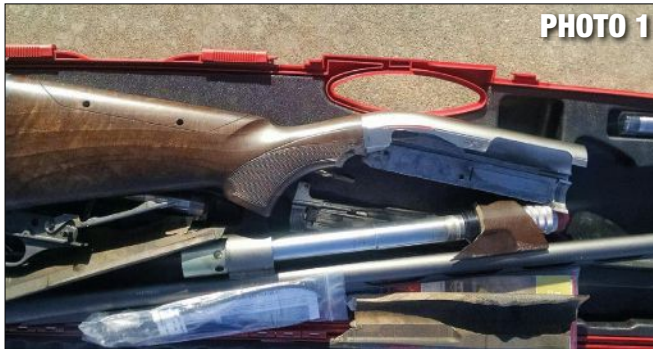
▼ Photo 1: A blown-out receiver and a shattered forend.
